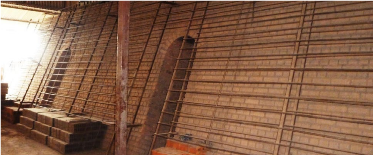
Former Amagerwa (Kigali, Rwanda) Ugandan kiln with average production capacity of 4 - 4.5 million bricks per year.
