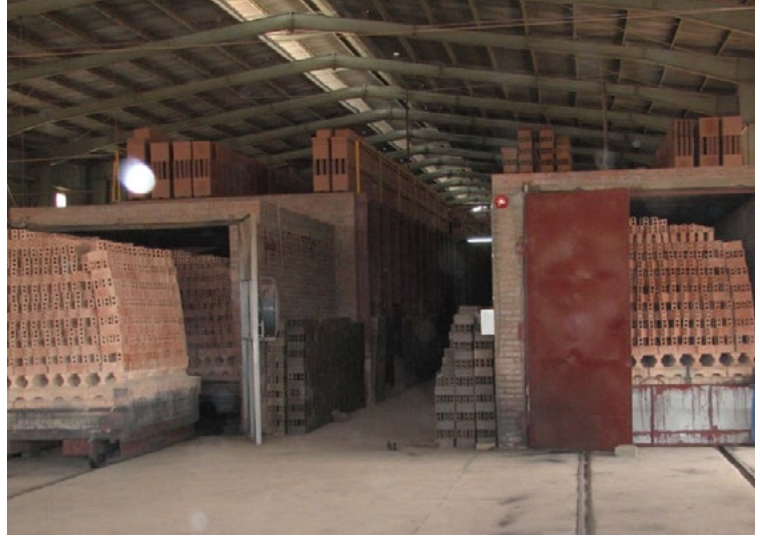
Top: Graphic illustration of tunnel kiln automated production cycle. Bricks are loaded on cars that are fed through a tunnel. Recycled heat from the kiln is pumped into a dryer to speed up the drying process. Bottom left: Inside a tunnel kiln with rails. Bottom right: Photo of tunnel kiln on the left and dryer with metal doors on the right.
