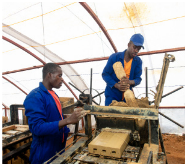
Locally-sourced manual machines are managed by mobile teams that can be deployed on a construction site.
