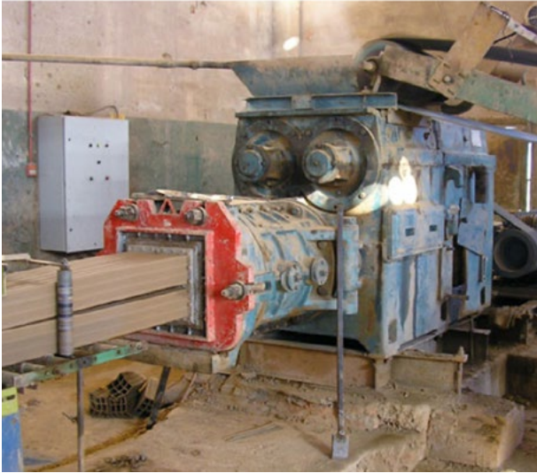
High-capacity mechanized extruder permits simultaneous extrusion of multiple products.
