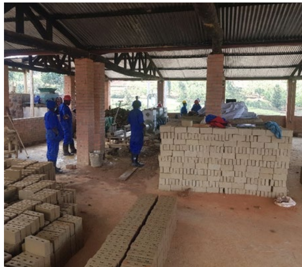
Large hangars are used to store products before firing. The hangars are designed to allow sufficient airflow to uniformly dry the products.
