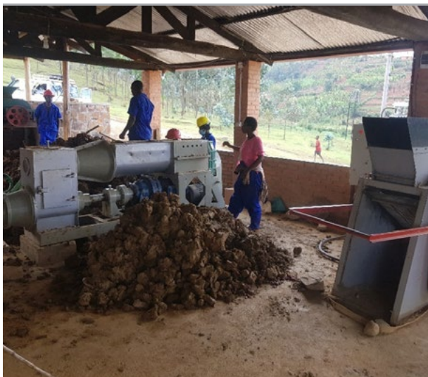
A small production line consists of a crusher and motorized extruder with vacuum pump.
